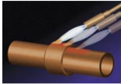
Bring both pieces being brazed up to temperature evenly and quickly
