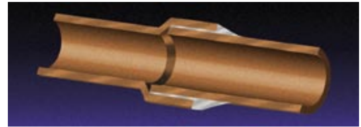
A well brazed joint – proper alloy flow reaches inside the joint
