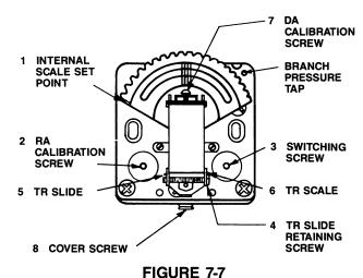
The 2230-018 Humidistat (figure 7-7) is factory set for a 10% throttling range, set in reverse action and calibrated for 9 psig when the ambient relative humidity equals the set point. It should not require calibration upon installation unless the throttling range is changed.
