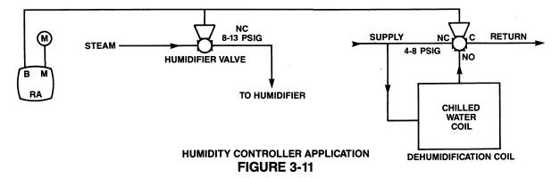
Figure 3-11 illustrates a humidistat application. The reverse acting humidistat is controlling a normally closed steam valve and 3-way chilled water valve. Hence, when the output pressure of the humidistat is between 8 and 13 psig, the normally closed steam valve is open and adding humidity to the system.
