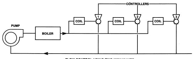
FLOW CONTROL USING TWO-WAY VALVES
