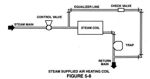
Figure 5-8 illustrates a steam-supplied air heating coil. The illustration shows the most favorable design conditions and piping arrangement that lends itself to good control valve performance. General rules for this requirement are as follows:
