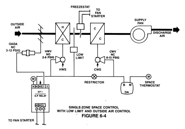
In this system (figure 6-4) the same function is being performed by the space thermostat as in the previously discussed singlezone system. However, additional controls that are often found in conjunction with the thermostat and coil controls in a system like this are added. This system also includes control of the outside air damper, the E-P relay that ties into the fan starter circuit to provide shutdown at night, and low-limit and freeze protection controls.
