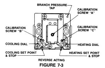
To calibrate the reverse acting models, refer to figure 7-3 and proceed with calibration as outlined under the procedures for the direct acting models.
