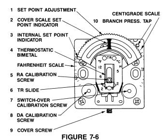
The 2218 (figure 7-6) is factory calibrated with the throttling range set at 3°F, and should not be recalibrated unless the throttling range is changed, or limited summer control action at 8 psig main pressure is required. If recalibration is required, proceed as follows:
