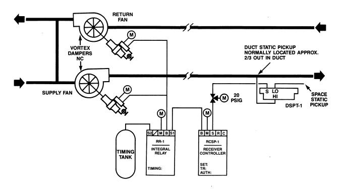
OPEN LOOP SUPPLY AND RETURN FAN CAPACITY CONTROL RESET FIGURE 6-26
