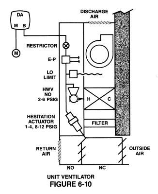
Figure 6-10 depicts a unit ventilator. The unit ventilator is a self-contained unit with the exception of a hot water supply from a central boiler. It does not rely on any central air handling system. It is generally located beneath the windows on an outside wall where the normally closed outside air dampers would bring in air for ventilation from the outside and the normally open return air dampers would be able to recirculate the return air after mixing it with the outside air.
