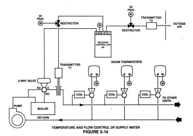
3) With average conditions, heating unit valves will be working near midstroke rather than operating as two-position between closed and nearly closed positions. A typical piping arrangement for temperature and flow control of supply water is shown in figure 5-14.
