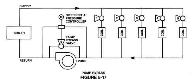
Many applications specify a pump bypass as shown in figure 5-17 to maintain a constant pressure across the system. As the control valves on the individual heating units decrease the flow through the system during low heat demand, pressure across supply and return mains increase. The increase in pressure is too high to allow accurate control by the unit valves.
