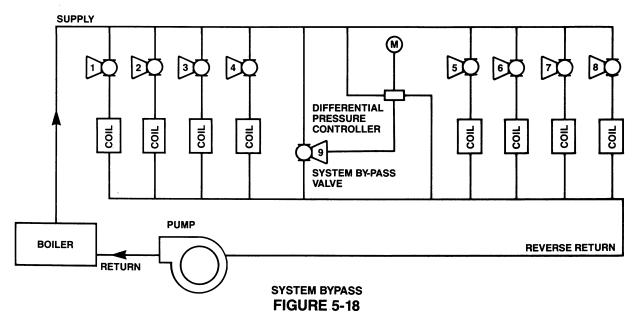
Another method of regulating system differential pressure is by using a system bypass valve as shown in figure 5-18. By placing
