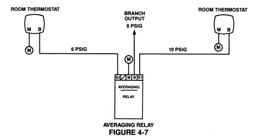
This type of relay is designed for use in pneumatic control systems where the application requires operation of a final control device by the average signal from two pneumatic controllers. In the example shown in figure 4-7 the two space thermostats send their
