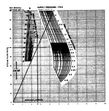
TO DETERMINE Cv: (1) Mark intersection of steam supply pressure (psig) and maximum allowable pressure drop (psi) within proper family of curves.
