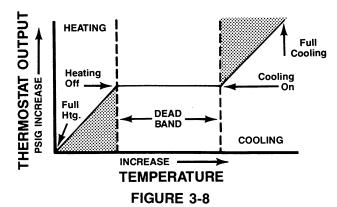
Figure 3-8 shows that the output of a direct acting thermostat rises to the dead band pressure. The dead band pressure is then maintained until the cooling set point is reached. At this point, the branch pressure will rise to main air pressure should the room temperature continue to rise.
