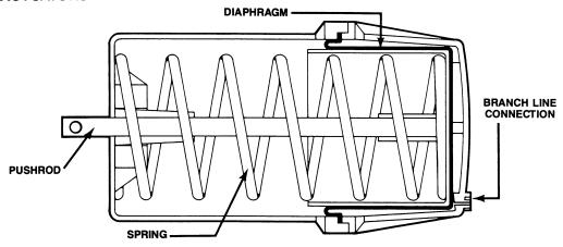
CUTAWAY OF DAMPER ACTUATOR FIGURE 5-3
